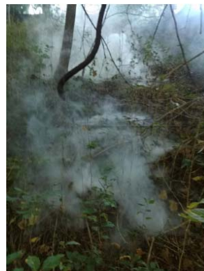
North Royal Ave. - Lateral Sewer Defect
