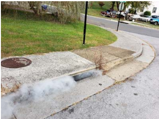
Hill Street - Smoke in Storm Inlet
