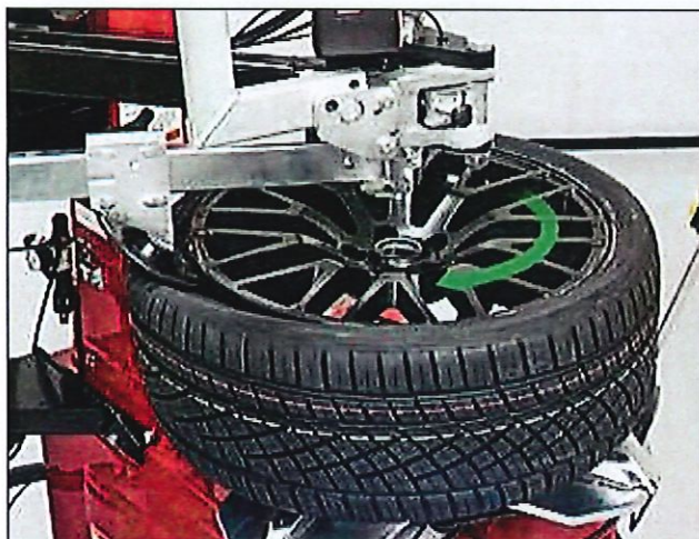
A single bead press roller disc can quickly assist mounting and demounting stiff sidewall tires.
