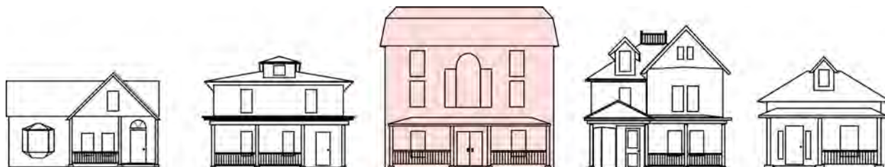
Figure 3-98: Inappropriate scale in red.
