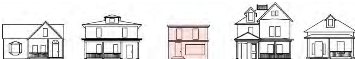
Figure 3-97: Inappropriate scale in red.
