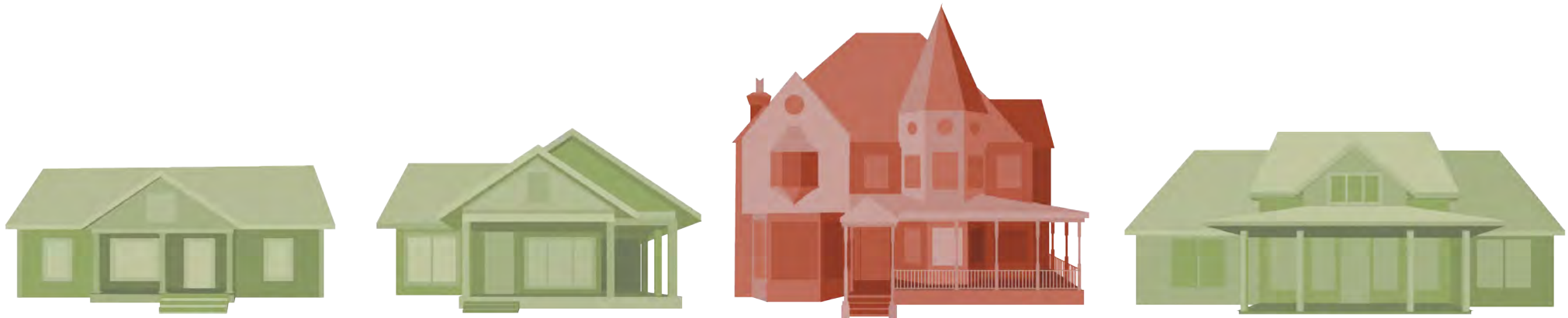
Figure 3-92: The building in red is an example of incompatible massing. All neighboring buildings have more simplistic windows, openings, rooflines, and other base architectural form.
